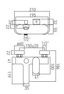
2 hole exposed bath shower mixer single lever wall mounted without shower kit ceramic cartridge CAR-K35B 1/2" x 3/4" x 50mm eccentrics minimum operating pressure 1.5 bar MP
