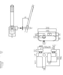
2 hole exposed bath shower mixer single lever wall mounted with shower kit ceramic cartridge CAR-K35B 1/2" x 3/4" x 50mm eccentrics minimum operating pressure 1.5 bar MP
