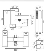
Té 2 hole bath shower mixer deck mounted with Mix<sup>2</sup> single function handset with water flow straightener cold ceramic cartridge C-302-RTC hot ceramic cartridge C-302-LTC 2 x 3/4" x 55mm fixed tails deck mount drill hole diameter 28-30mm minimum operating pressure 0.2 bar LP
