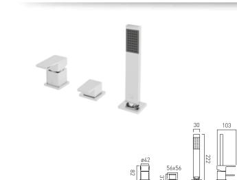
3 hole bath shower mixer single lever deck mounted without spout with shower kit for use with bath filler waste and overflow ceramic cartridge SYN-CARTRIDGE/B diverter cartridge CAR-KD235A minimum operating pressure 3.0 bar HP chrome SYN-132/NS-C/P Stocked In UK
