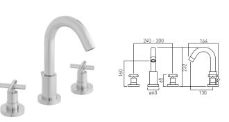
3 hole basin mixer with swivel spout deck mounted with pop-up waste with water flow aerator cold ceramic cartridge C-206-RTC hot ceramic cartridge C-206-LTC 2 x 1/2" nut x 600mm flexipipe connections valve deck mount drill hole diameter 27mm spout deck mount drill hole diameter 30mm minimum operating pressure 0.2 bar LP chrome ELW-101-C/P Stocked In UK
