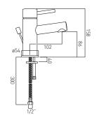
mono basin mixer single lever deck mounted with pop-up waste with water flow aerator ceramic cartridge CAR-K40A deck mount drill hole diameter 35mm minimum operating pressure 0.2 bar LP Stocked In UK / Dubai
