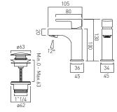
single lever deck mounted smooth bodied with universal basin waste with directional water flow aerator ceramic cartridge LIF-100M-CAR 2 x 1/2" x 400mm flexipipe connections deck mount drill hole diameter 35mm minimum operating pressure 0.5 bar LP
