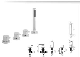
4 hole bath shower mixer deck mounted with shower kit without spout for use with bath filler waste and overflow cold ceramic cartridge C-303-RTC hot ceramic cartridge C-303-LTC diverter cartridge ELE-DIVERTER/D-CART 2 x 3/4" x 3/4" x 600mm flexipipe connections valve deck mount drill hole diameter 33mm diverter deck mount drill hole diameter 46mm handset deck mount drill hole diameter 27mm minimum operating pressure 1.0 bar MP
