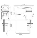
mono basin mixer single lever deck mounted with pop-up waste with water flow aerator with water flow straightener ceramic cartridge CAR-K40B 2 x 1/2" nut x 300mm flexipipe connections deck mount drill hole diameter 35mm minimum operating pressure 0.2 bar LP
