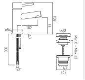
mono basin mixer single lever deck mounted smooth bodied with universal basin waste with water flow aerator ceramic cartridge CAR-K40A deck mount drill hole diameter 35mm minimum operating pressure 0.2 bar LP
