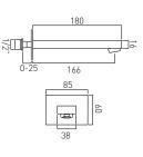
bath spout wall mounted 1/2" inlet min-max wall mount 0-25mm minimum operating pressure 0.2 bar LP chrome NOT-140-C/P Stocked In UK / Dubai
