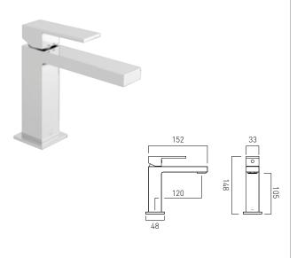
single lever deck mounted smooth bodied without universal basin waste with water flow aerator ceramic cartridge C-010-N25 2 x 1/2" nut x 400mm flexipipe connections deck mount drill hole diameter 35mm minimum operating pressure 1.0 bar MP
