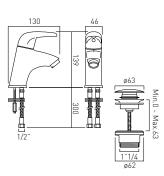
mini mono basin mixer single lever deck mounted smooth bodied with universal basin waste with water flow aerator ceramic cartridge CAR-K35B 2 x 1/2" nut x 400mm flexipipe connections deck mount drill hole diameter 35mm minimum operating pressure 0.2 bar LP
