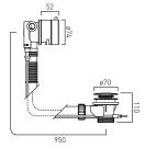
pop-up bath filler waste and overflow 2 x 1/2" inlets (one is blanked off) 1.1/2" x 10mm threaded outlet connection min-max overflow bath thickness 1mm-11mm minimum operating pressure 1.0 bar MP
