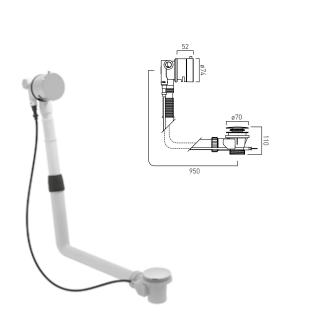
pop-up bath filler waste and overflow 2 x 1/2" inlets (one is blanked off) 1.1/2" x 10mm threaded outlet connection min-max overflow bath thickness 1mm-11mm minimum operating pressure 1.0 bar MP
