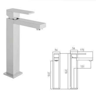
extended mono basin mixer single lever deck mounted smooth bodied without universal basin waste with water flow aerator ceramic cartridge CAR-K28A 2 x 1/2" nut x 550mm flexipipe connections deck mount drill hole diameter 35mm minimum operating pressure 1.0 bar MP
