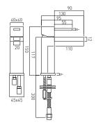
mono basin mixer with waterfall spout single lever smooth bodied without universal basin waste ceramic cartridge CAR-K28A 2 x 1/2" x 400mm flexipipe connections deck mount drill hole diameter 35mm minimum operating pressure 0.2 bar LP
