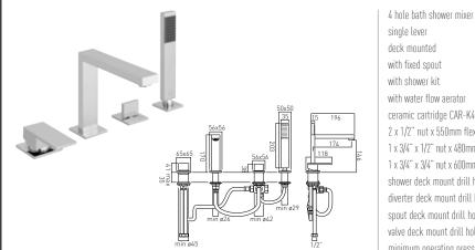
single lever deck mounted with fixed spout with shower kit with water flow aerator ceramic cartridge CAR-K40A 2 x 1/2" nut x 550mm flexipipe connections 1 x 3/4" x 1/2" nut x 480mm flexipipe connection 1 x 3/4" x 3/4" nut x 600mm flexipipe connection shower deck mount drill hole diameter 30mm diverter deck mount drill hole diameter 42mm spout deck mount drill hole diameter 26mm valve deck mount drill hole diameter 45mm minimum operating pressure 3.0 bar HP
