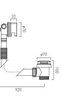
push type bath filler waste and overflow 2 x 1/2" inlets (one is blanked off) 1.1/2" x 10mm threaded outlet connection min-max overflow bath thickness 1mm-21mm minimum operating pressure 1.0 bar MP
