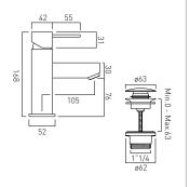
mono basin mixer single lever deck mounted smooth bodied with universal basin waste with water flow aerator ceramic cartridge CAR-K35A 2 x 1/2" x 400mm flexipipe connections deck mount drill hole diameter 35mm minimum operating pressure 0.2 bar LP
