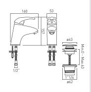
single lever deck mounted smooth bodied with universal basin waste with water flow aerator ceramic cartridge CAR-K40B 2 x 1/2" nut x 400mm flexipipe connections deck mount drill hole diameter 35mm minimum operating pressure 0.2 bar LP
