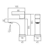
mini mono basin mixer single lever deck mounted smooth bodied without universal basin waste with directional water flow aerator ceramic cartridge LIF-100M-CAR 2 x 1/2" x 400mm flexipipe connections deck mount drill hole diameter 35mm minimum operating pressure 0.5 bar LP
