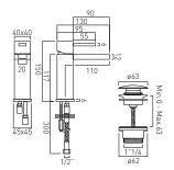
mono basin mixer with waterfall spout single lever smooth bodied with universal basin waste ceramic cartridge CAR-K28A 2 x 1/2" x 400mm flexipipe connections deck mount drill hole diameter 35mm minimum operating pressure 0.2 bar LP
