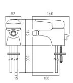
mono bidet mixer single lever deck mounted with pop-up waste with water flow aerator with water flow straightener ceramic cartridge CAR-K40B 2 x 1/2" nut x 300mm flexipipe connections deck mount drill hole diameter 35mm minimum operating pressure 0.2 bar LP
