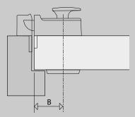
When selecting a replacement nightlatch, it is important to check that the backset (B) (ie. the measurement from the centre of the keyhole to the edge of the door) is the same as your existing lock. If you are fitting a lock to a new door, choose the longest backset that allows a comfortable fit.
