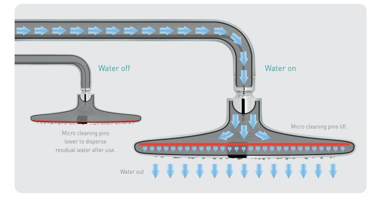
Integral to the shower head and handset is a system of micro cleaning pins designed to prevent residual water after use and stop subsequent limescale accumulation.
